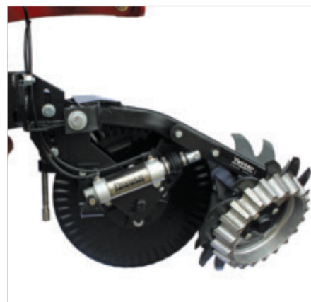
2x2 Fertilizer Row Opener • No-till floating dual wheel residue managers • Standard in-cab air control • Injector-style applicator
