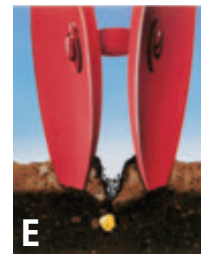
E Closing Disks OR V-wheel – Confirm covering disk action and seed trench closure ( E ).
