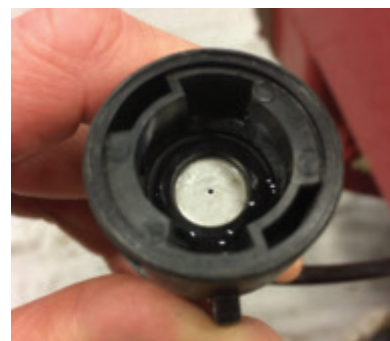
New for 2017: agitation nozzle at tank bottom
