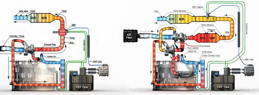
System component size varies from one machine application to another. Component sizes shown here are approximate and not to scale.
