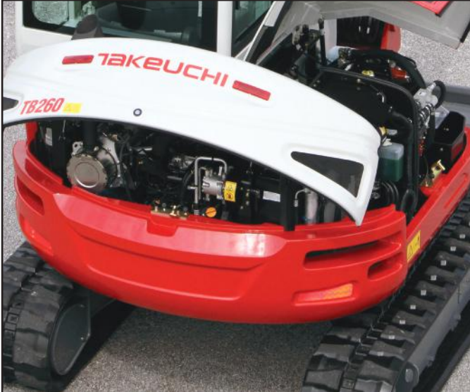
Large doors provide easy access to all major engine and hydraulic components.
