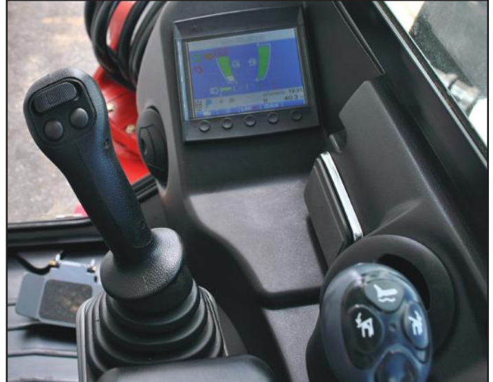
Low effort pilot controls and simple switches are easy to use.
