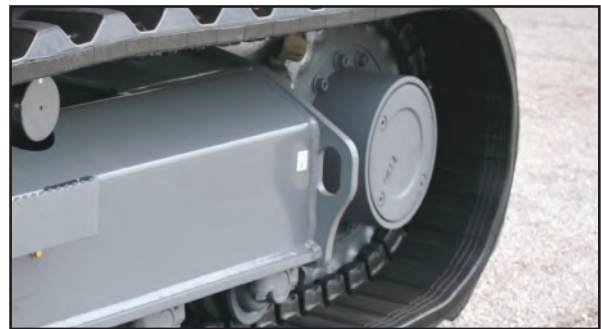
Two-speed travel with automatic shift down for turning and ascending grades.
