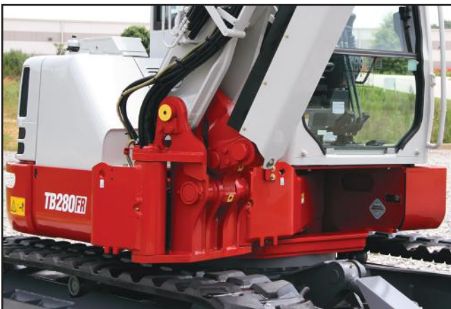
Unique Side-to-Side (STS) boom design enables this machine to work in confined work spaces.
