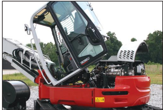
Tilt-up operator's platform provides improved access to all major hydraulic components.
