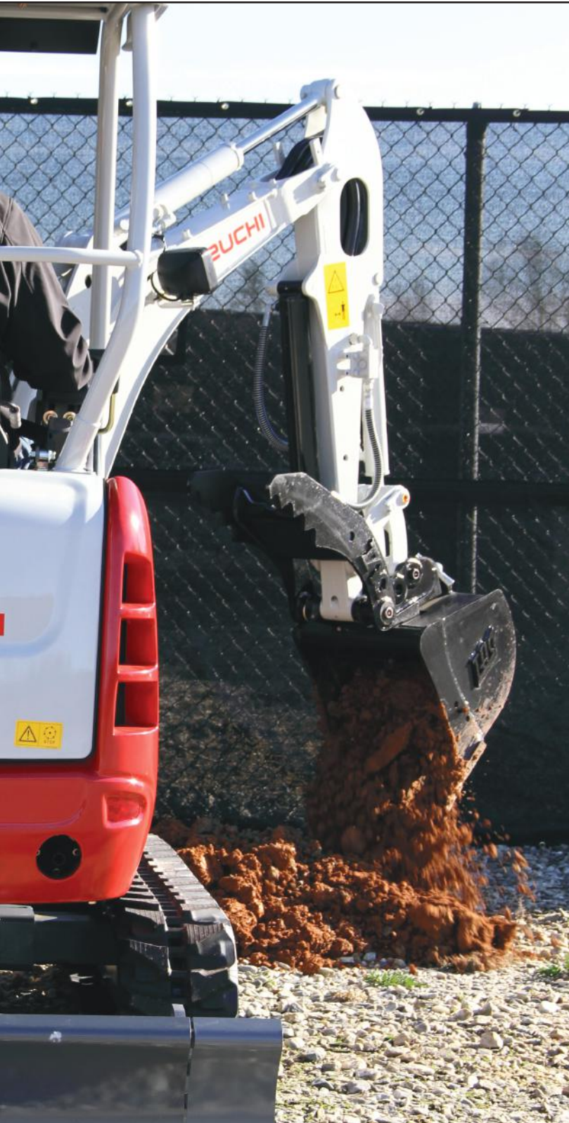
Standard long arm allows for greater reach and less time repositioning.
