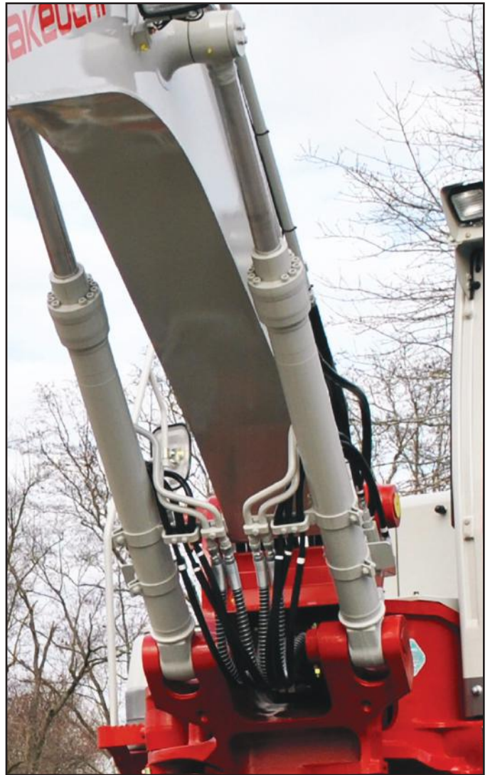
Two boom cylinders provide the strength needed for lifting, while the independent boom swing allows both excavators to dig offset over the left or right track.
