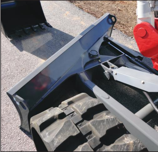
Heavy duty dozer blade with integrated anchor points.
