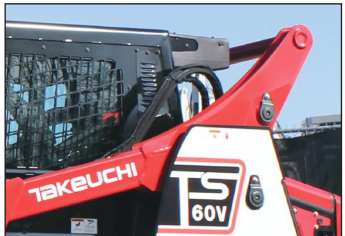
The low profile A/C system helps protect the unit from damage without blocking critical sight lines.
