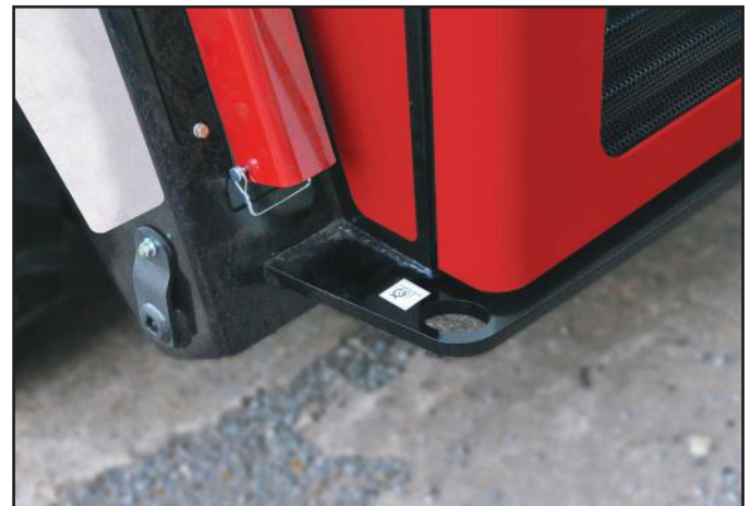
The large rear bumper provides protection for the rear of the machine and the large anchor points make it easy to secure the machine for transport.
