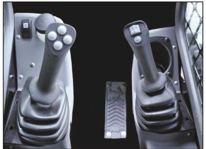
Low effort pilot controlled joysticks are responsive while the foot throttle helps to improve the efficiency of the machine.
