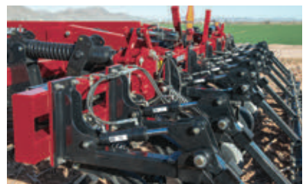
Crumbler pressure: achieve consistent clod sizing
