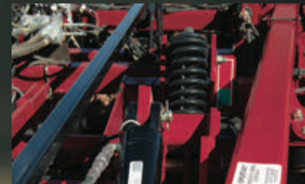
Disk gang pressure: reduce pressure on frame
