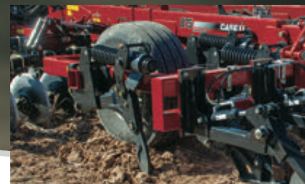
Shank depth: target the compaction layer
