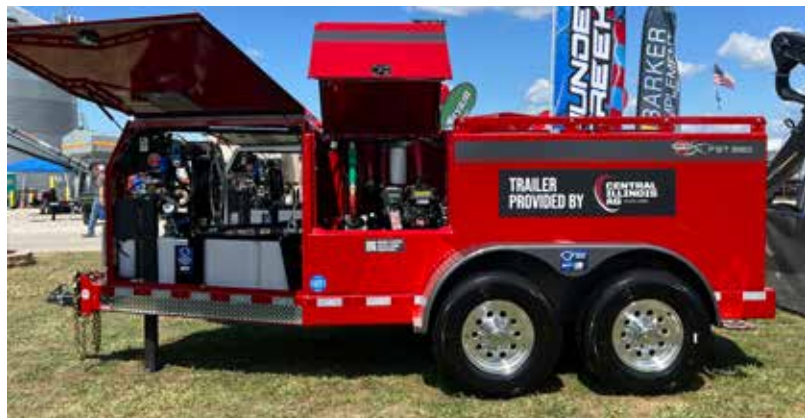
Photo (above): Thunder Creek FST990 without a rear utility box with the axle closer to the front of the trailer.
